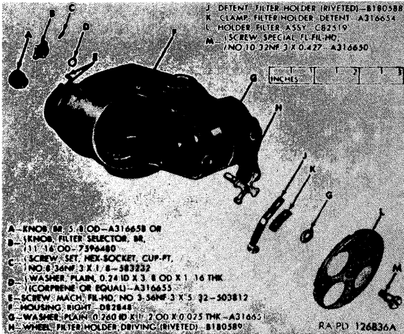
Figure 149. Right housing with filter holder assembly D74392 - exploded view.
